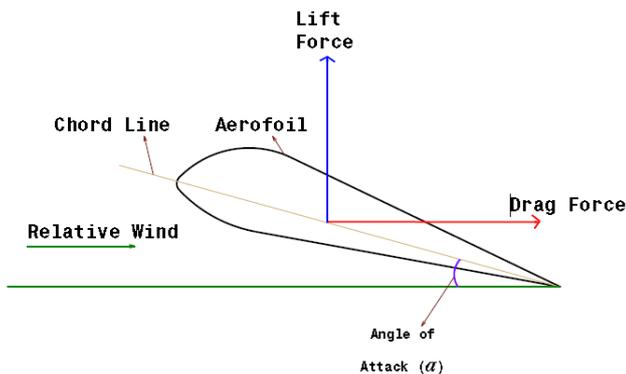
Fig. 2 : Lift and Drag Force
