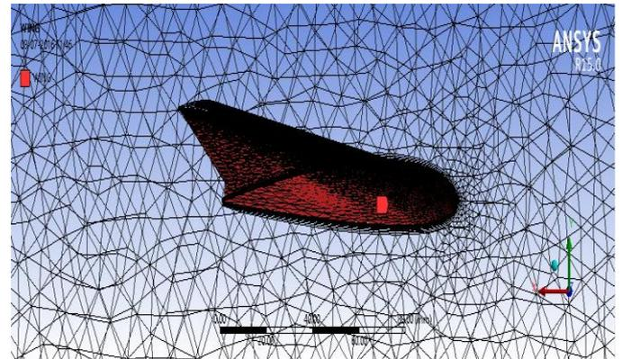
Fig.5 : 3-D Model of Wing with Meshing
