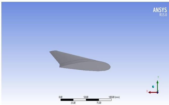
Fig.3 : Wing with NACA 2415
