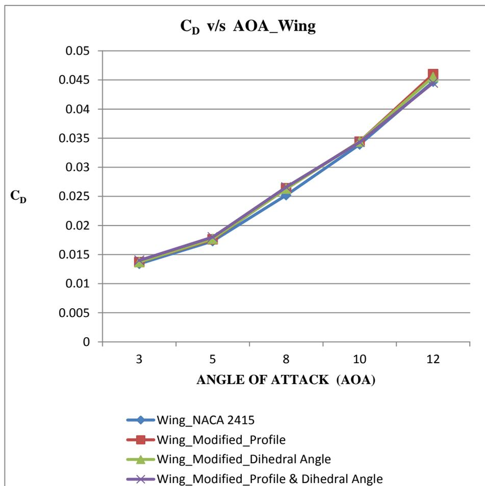
**Fig.7 : Drag Coefficient ( $C_D$ ) at various angle attack**
