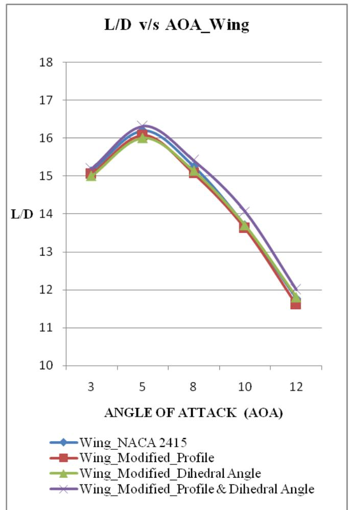
**Fig.8 : L/D Ratio at various angle attack**
