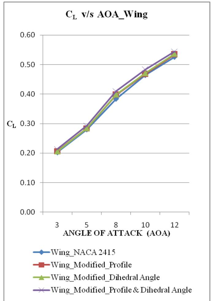
**Fig.6 : Lift Coefficient (C<sub>L</sub>) at various angle attack**
