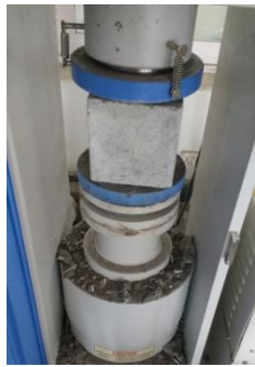
Fig -2 Compressive test on cube
