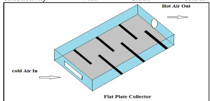
Collector plate is made up of glass which can be use for trapping the solar radiations. The blower is used to suck air from atmosphere and circulate hot air from the collector to the bed.
