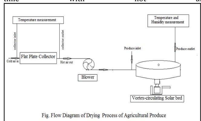
Fig. Flow Diagram of Drying Process of Agricultural Produce
