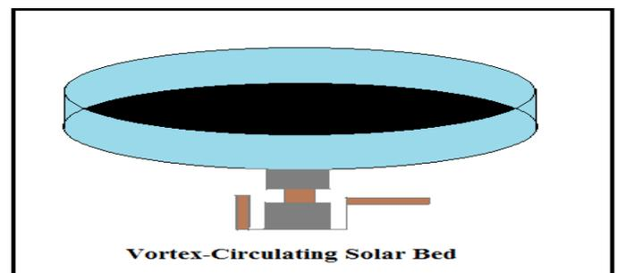
The chillies are fed in the bed and are spread over the bed as a thin layer due to bed circulation. The advantage of the vortex circulating bed is to provide constant movement of the chillies over the bed in order to enhance the resident time with hot air.
