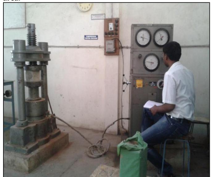
**Figure 1:** Experimentel setup of compression testing machine
