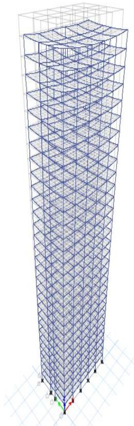
Fig 1: Deformed shape of structure after analysis
