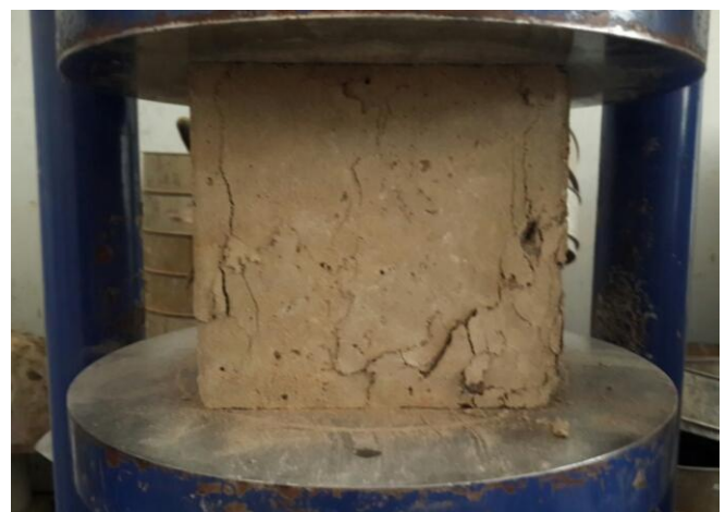
Fig -2: Testing of compressive strength test specimen
