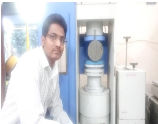
Fig -3: Testing of tensile strength test specimen
