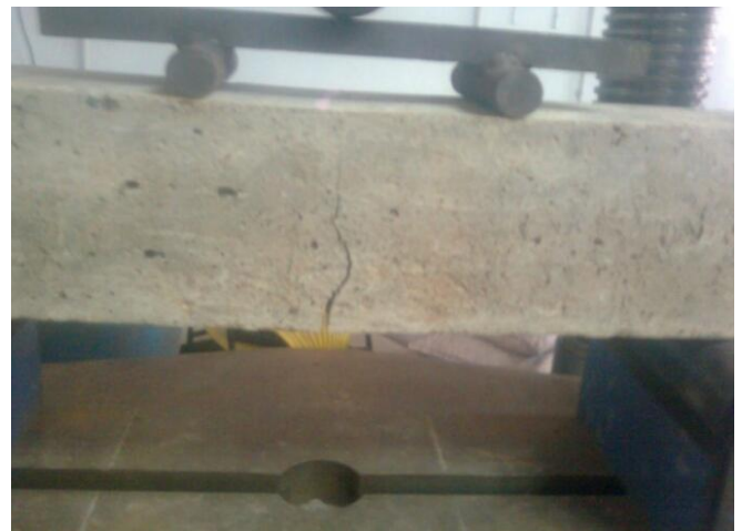
Fig -4: Testing of flexural strength test specimen
