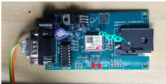
**Fig -7:** GSM Module
