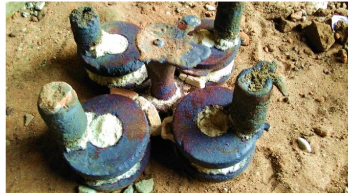
Fig.10 Castings after Shakeout operation
