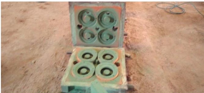
Fig.8 Cope and drag molding box assembly
