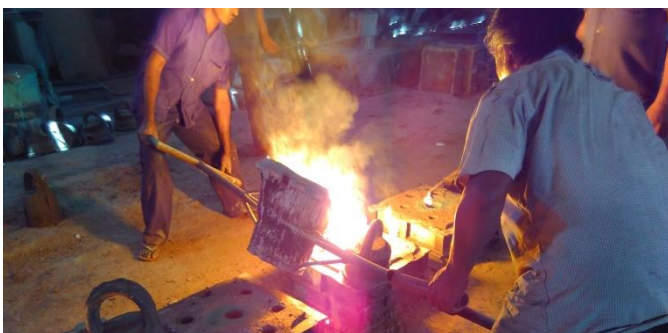
Fig.9 Melting and pouring using shank ladle
