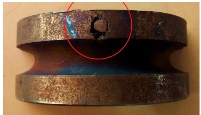
Fig.3 Shrinkage defect over pulley
