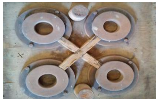
Fig.6 Cope portion of wooden pattern
