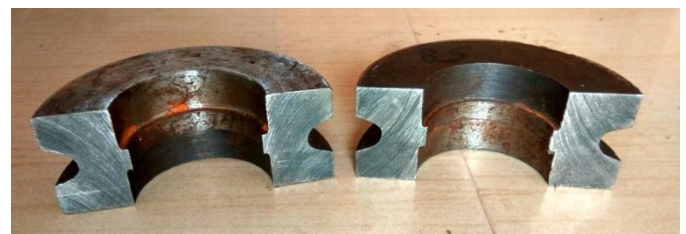
Fig.11 Casting sliced mechanically to locate internal void
