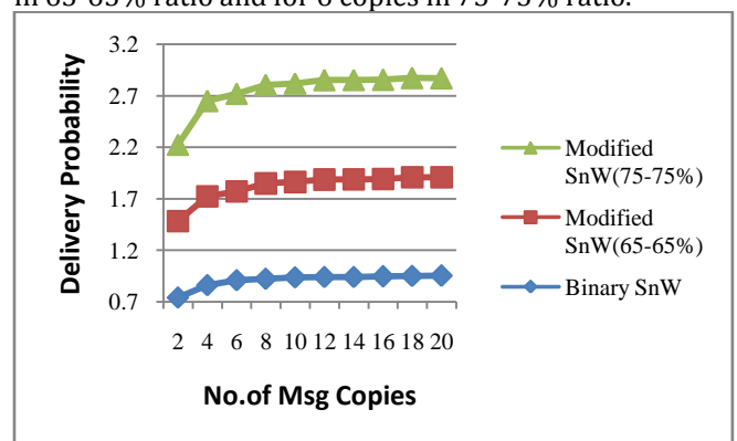
Fig-5: Delivery Probability vs. No. of Msg copies graph for comparison between existing Binary spray and wait and Modified Spray and wait protocols
