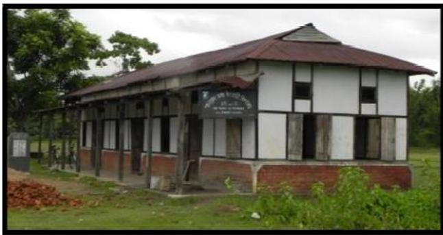
Figure 2:- Assam type roof (Light in weight)
