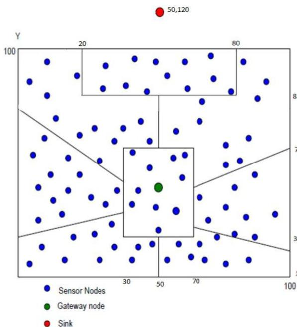
We placed sink node or base station far from sensing field and after placement sink node and sensor nodes both become stationary. A gateway node is also deployed at the middle of sensing field. After deployment gateway node is stationary and rechargeable. In proposed protocol we use homogeneous nodes, which have same computational & sensing capability. An ID (distinctive identifier) is assigned to each sensor node.
