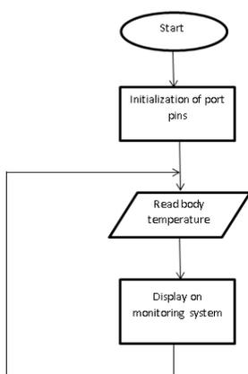
Figure 5.1 flow chart that detects body temperature.
