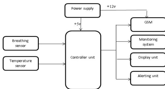
**Figure 3.1** system block diagram of Non-Invasive Sleep Apnea Detection System for Continuous monitoring during daily life
