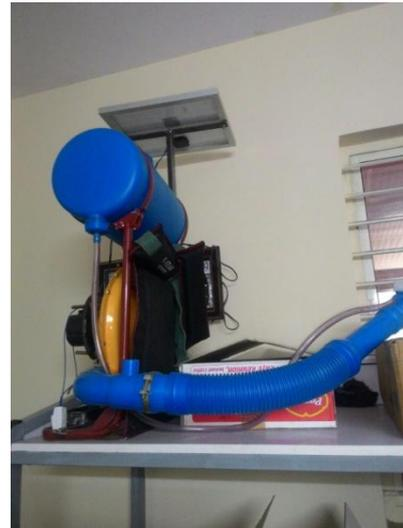
Figure 3: Working model of multiple power supplied fertilizer sprayer
