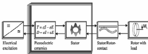
Fig- 5: Working of Piezoelectric motor.
