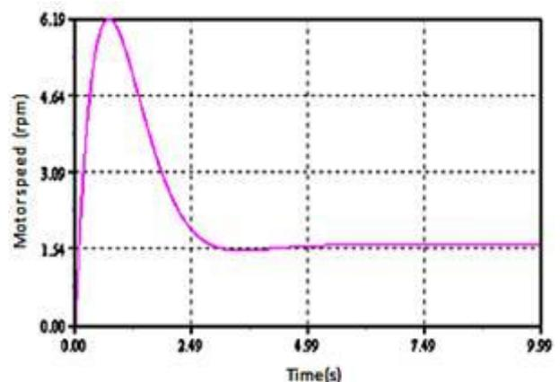
Chart -2: Motor speed as a function of time for a load of 3N.
