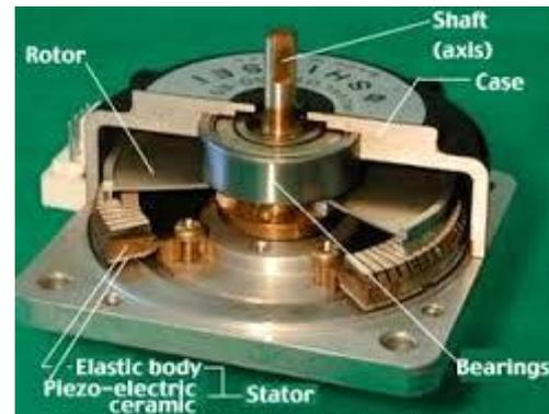
Fig- 3: Piezoelectric motor
