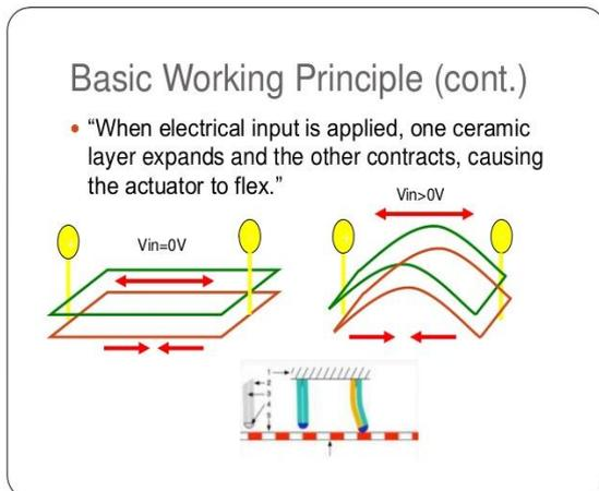
Fig- 2: working principle of Piezoelectric motor.
