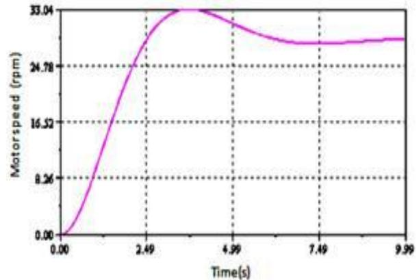
Chart -1: Piezoelectric motor speed without load.
