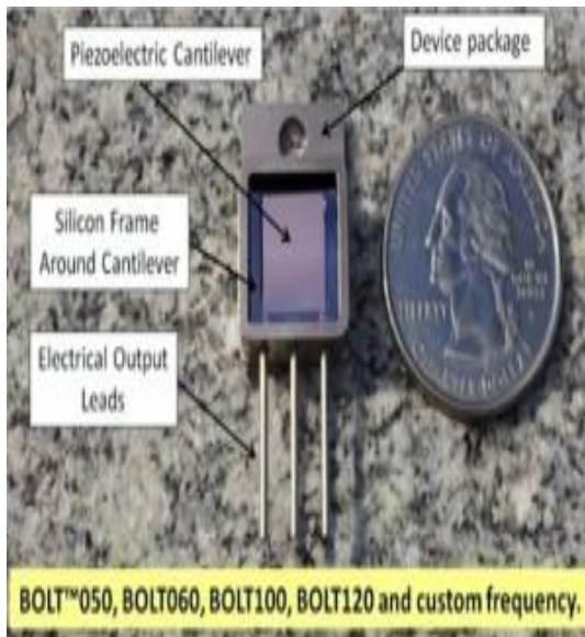
Fig -4: Smart dust internal structure
