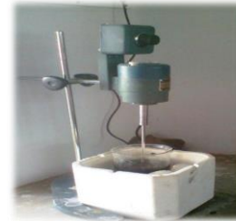
Fig.2.2 Polymer preparation Setup
