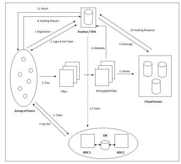
Fig -1: System Architecture
