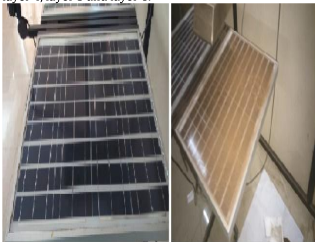
Fig. 1 - Clean solar panel and dust deposited solar panel
