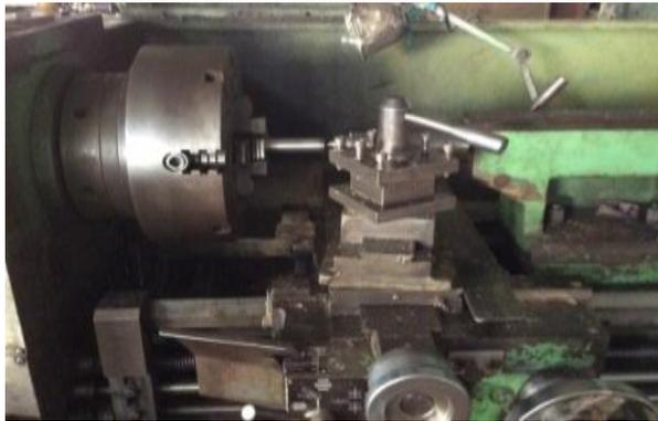
Fig.1: Center drilling of work piece
