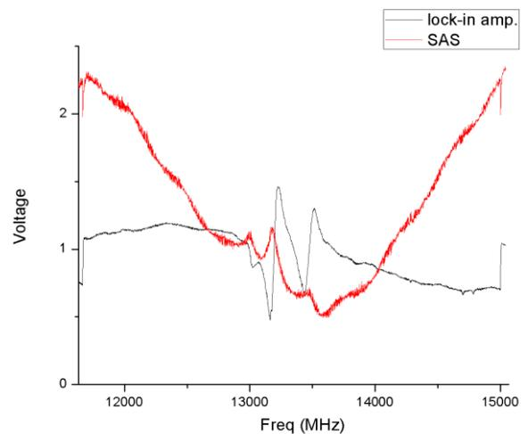
Fig 3.1 Output of SAS and lock in amplifier
