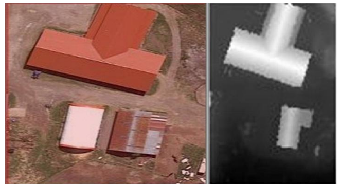
Figure2. (a) Digital map of area from where the Lidar is collected, (b) the corresponding DSM model generated.
