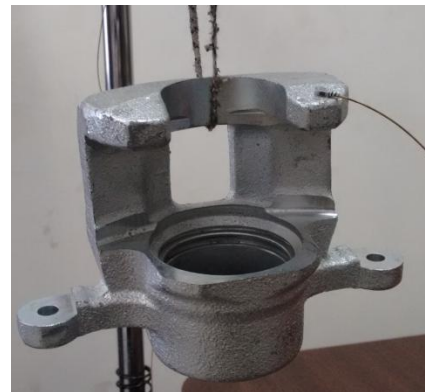
Fig-2: (Accelerometer location on caliper with free hanging condition )
