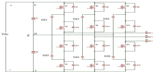
Figure.1 Three Level NPC Inverter (10)
