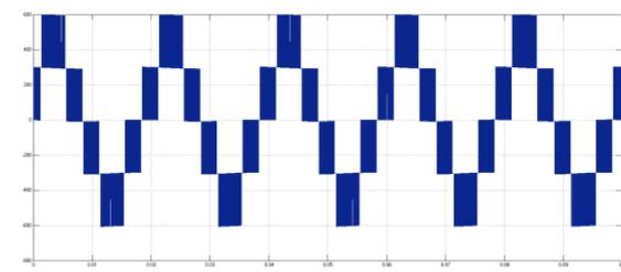
Figure.6 Waveform Of Line Voltage
