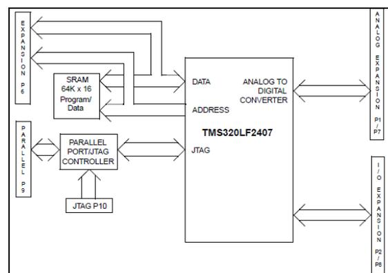
Figure.3 Block diagram OF eZdsp™LF2407
