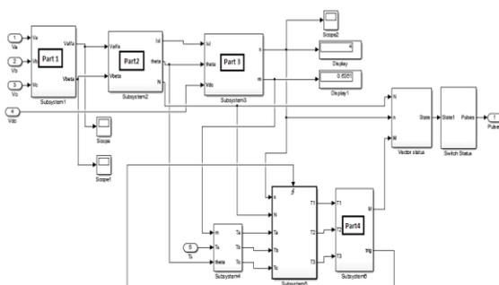
Figure.4 Overview Of Three Phase Three Level SVPWM Inverter Made In Simulink And Different Calculating Part
