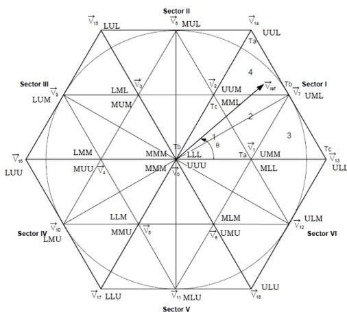
Figure.2 Space Vector Diagram of 3 Level Inverter
