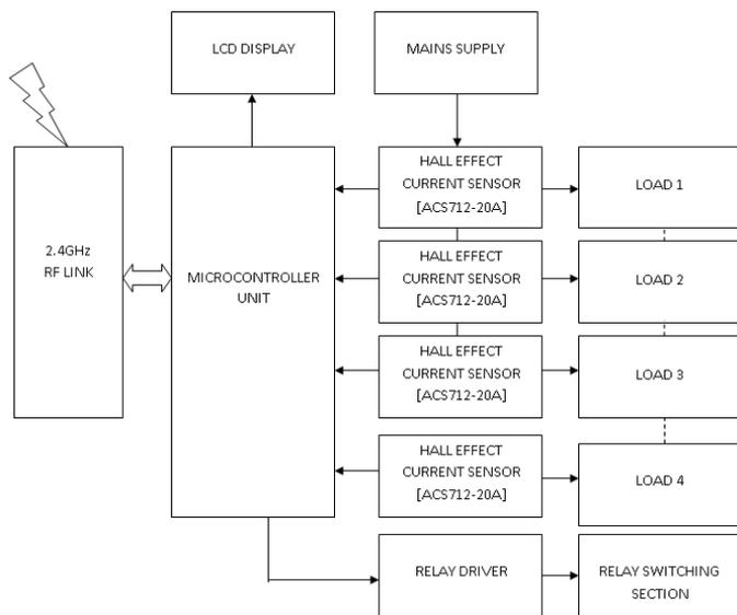
Fig -1: Sensing Unit Block Diagram
