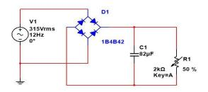
Fig-5: Power harvesting circuit
