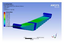
Fig-2:Stresses developed in spring steel leaf spring
