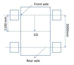
Fig-1:Schematics of vehicle for load calculations
