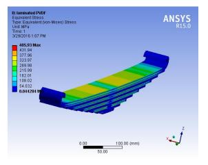
Fig-4:Stresses developed in spring with PVDF
