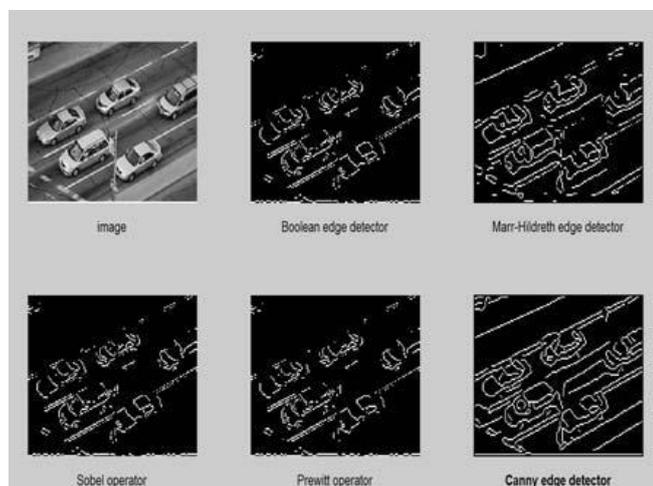
Fig- 3: Edge based Object detection
