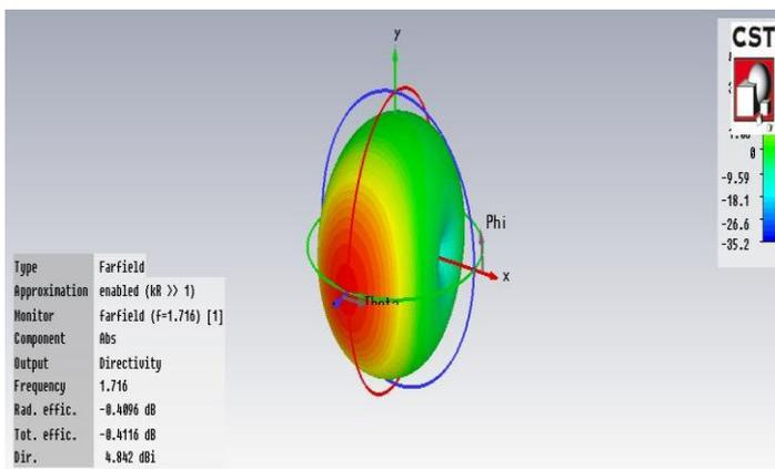
**Fig. 5:** Radiation pattern of RMPA shows directivity 4.842 dBi
