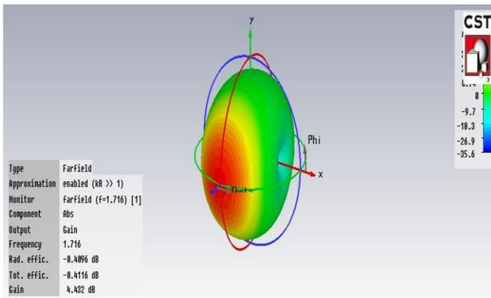
**Fig. 4:** Radiation pattern of microstrip antenna shows gain and total efficiency
