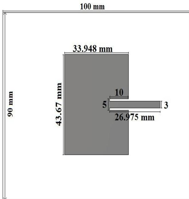
**Fig. 1:** Microstrip Rectangular patch antenna at 1.716 GHz (all dimensions are in millimeter)
