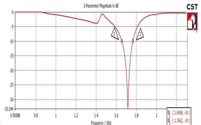
**Fig. 3:** Result of antenna show Return Loss of -33.24 dB and bandwidth of 109.4 MHz.
