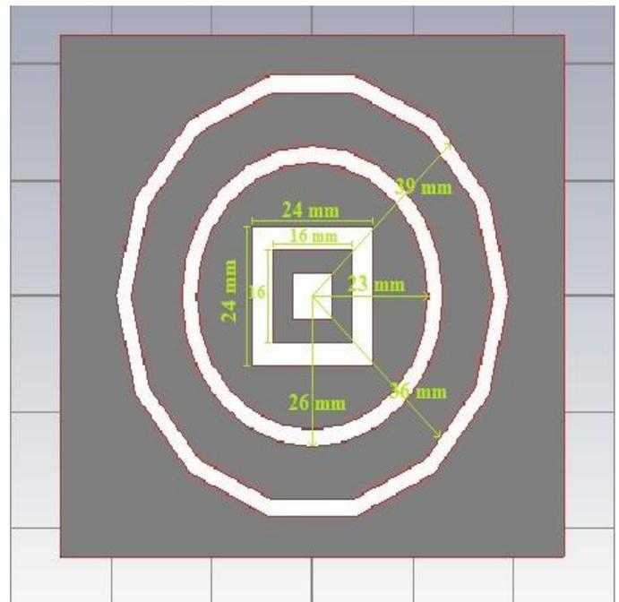
**Fig. 2:** Discontinuities at ground structure of rectangular patch antenna (all dimensions are in millimeter)
