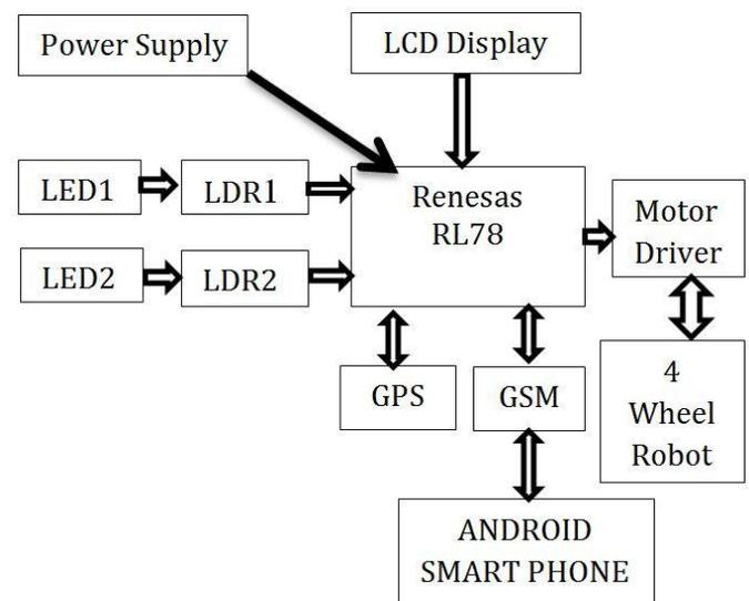
Fig -2: Robust Railway Track Crack Detection Scheme
