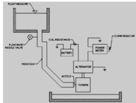
The layout of a common Pico hydro power plant is given by the above figure. The various components used in Pico hydro power plant are the reservoir, penstock, nozzle, turbine, alternator, battery and net meter. Reservoir is used to store the water and is supplied to the turbine through the pen stock through the vent. The flow of water is controlled with the help of valve. The turbine rotates due to force of water which due to which the turbine rotates.
