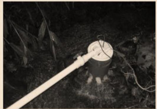
Pen stock is a narrow pipe like structure that connects reservoir to the turbine. Heavy water flows from the reservoir to the turbine through the pen stock. Due to the force of water the turbine blade rotates which further rotates the shaft at a high speed which is connected to the generator, which produces the electrical power.
