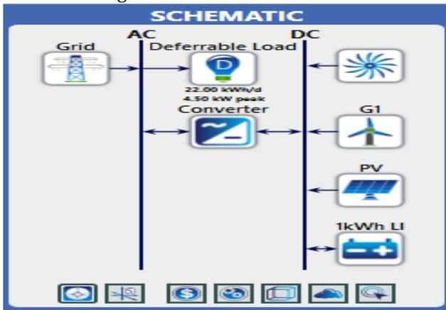
The above Diagram shows the connection of hydro power plant along with other sources of power in Green Building, which are solar power (PV cells), Wind turbine, Battery banks and the Grid.
