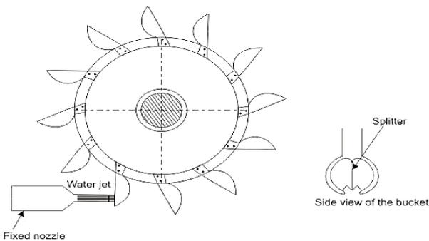
Turbine is a device that converts the potential energy of water to the mechanical energy which is converted to electrical energy with the help of generator.
