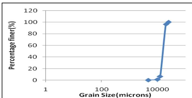
Chart -1: Particle Size Distribution Graph for Coarse Aggregates
