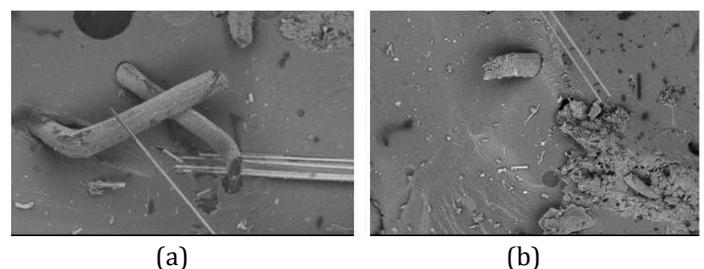
**Fig -3:** Scanning electron micrographs of coir/glass fibre reinforced epoxy composite specimens after tensile test
