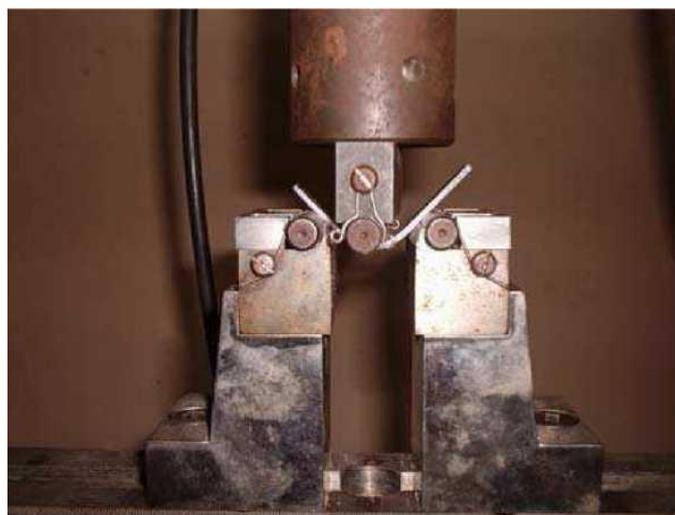
Fig -2: Loading arrangement for flexural test
