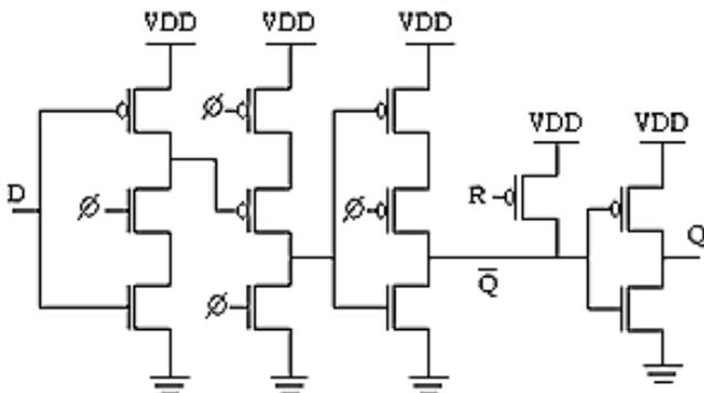
Fig-7: Negative Edge Trigger TSPC Flip-Flop
