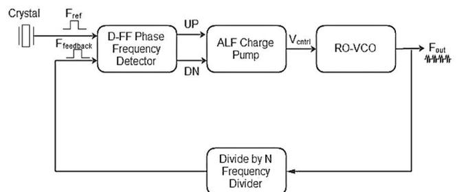
Fig -2: Block Diagram of Modified PLL
