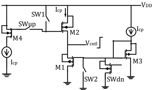
Fig -3: Schematic of MSCC Charge Pump
