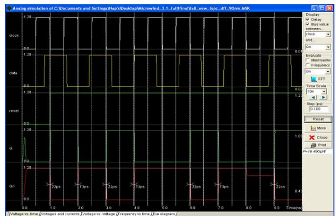
Fig-9: Simulation of D-FF TSPC Flip-Flop in Microwind
