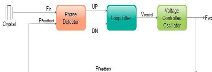
Fig -1: Block Diagram of Traditional PLL
