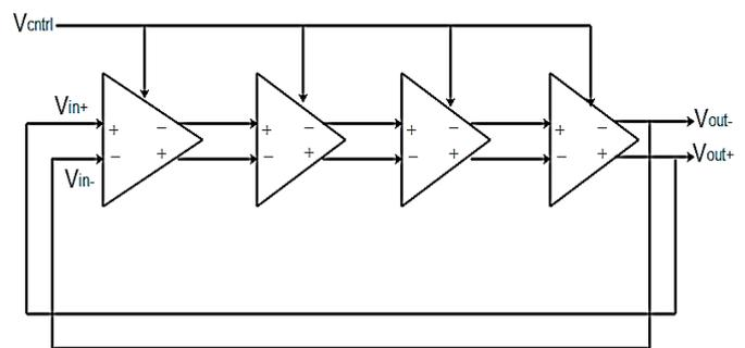
Fig -4: 4-stage Delay Cells in RO
