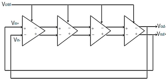
Fig -4: 4-stage Delay Cells in RO
