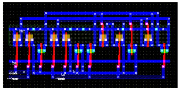
Fig-8: Layout of D-FF TSPC Flip-Flop in Microwind
