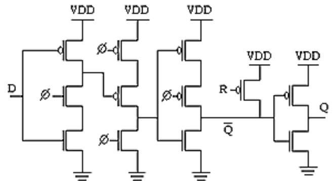
Fig-7: Negative Edge Trigger TSPC Flip-Flop
