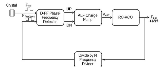
**Fig -2:** Block Diagram of Modified PLL
