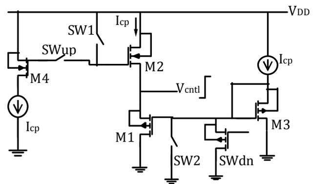
Fig -3: Schematic of MSCC Charge Pump
