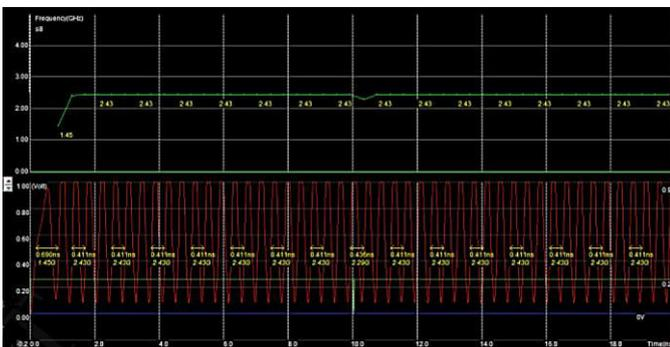
Fig -6: Simulation of LV-Ring VCO in Microwind
