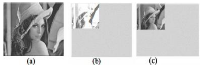
Fig -1: (a) Original image Lena. (b) One level DWT in sub band LL (c) One level IWT in Sub-band LL.
