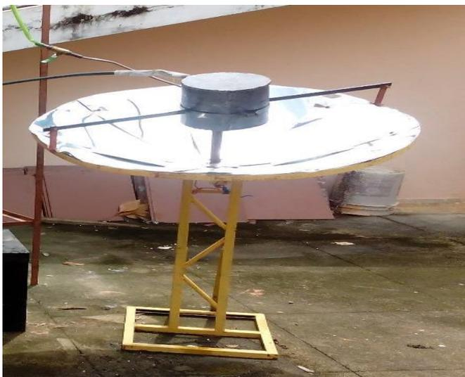
Fig -1: Parabolic dish collector
