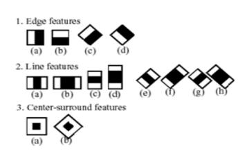
These are composed of either 2 or 3 rectangular sections. Face Candidates are scanned and searched for Haar features of the current stage. The weights are constants. Weights are generated by the learning algorithm.
