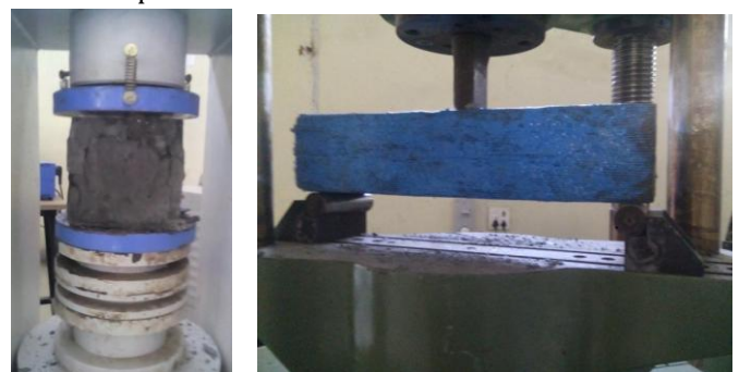
Photo.1: Test setup and instrumentation of beam
