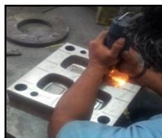
**Fig 10. Polishing Process**
