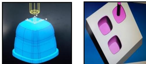
**Fig 3. Core and cavity on DELCAM software**
