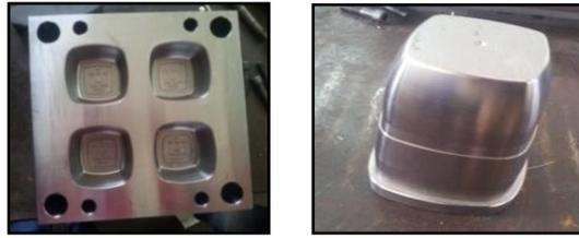
**Fig 11.cavity and core after machining process**
