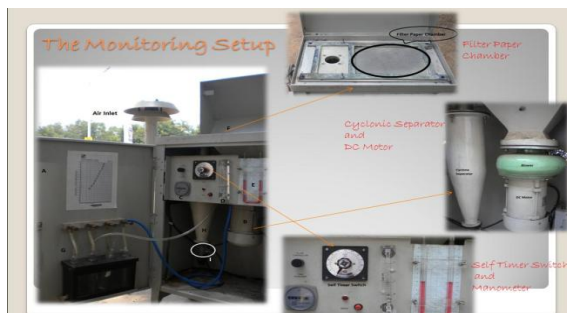
Fig-2: Showing details of HVS apparatus
