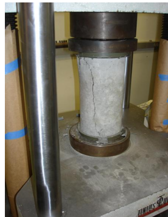
Fig 2: compressive strength test
