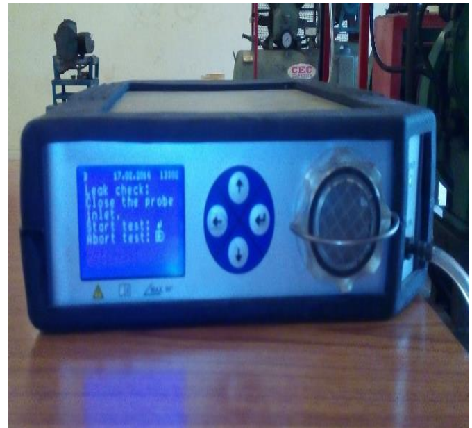
Fig- 6: Photographic View of the AVL Exhaust Gas Analyzer
