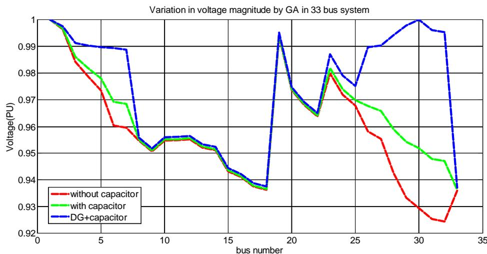
**Figure 1:** Variation in voltage magnitude by GA in 33 bus system
