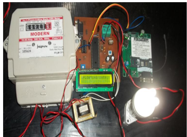
Fig -5: Automatic Energy Meter system
