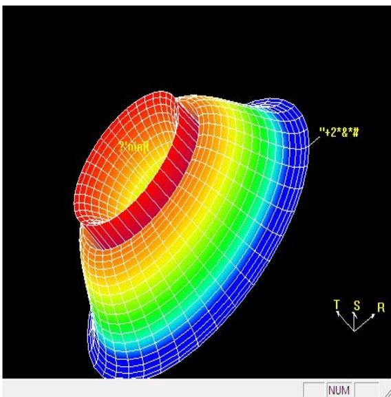
Fig.7. 3D Radiation Pattern of Praposed Antenna
