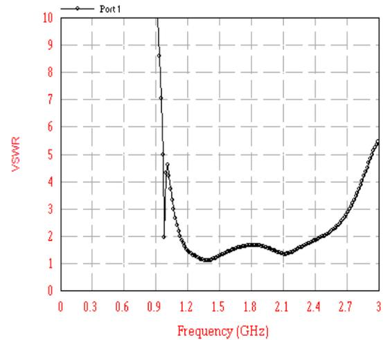
Fig.4. VSWR vs Frequency of Proposed antenna
