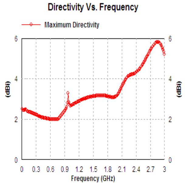
Fig.8. Directivity vs frequency graph
