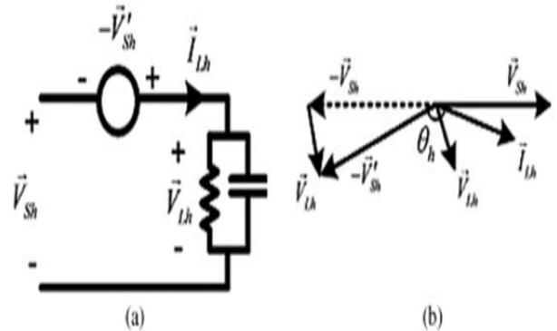
**Fig 3:** Sensitive Load SC Branch (a) Equivalent Load describing Harmonic Compensation in practice (b) Phasor Diagram for the hth harmonic order
