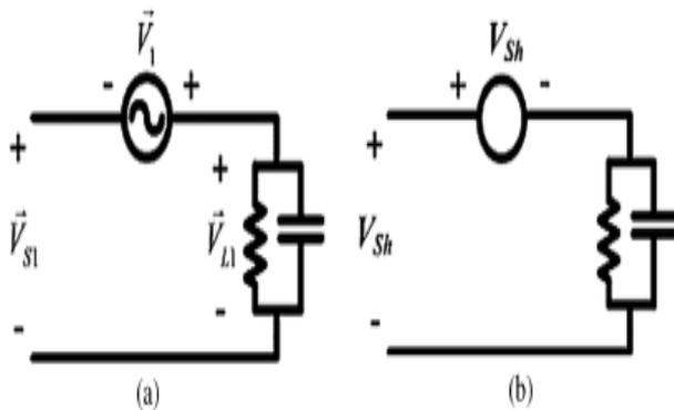
**Fig 2:** Equivalent Circuits of the Sensitive Load-SC branch for (a) Fundamental Component (b) hth Harmonic Component
