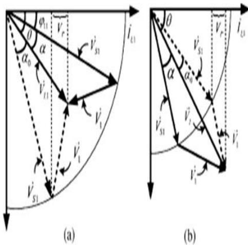
**Fig 4:** Phasor Diagram showing Voltage Restoration during (a) Voltage Swell (b) Voltage Sag : Fundamental Frequency Component
