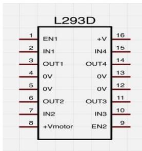
Fig-3: PIN configuration of L293D
