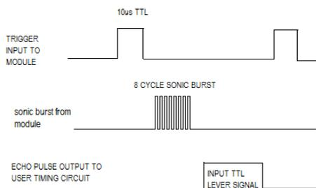
Fig-4: Timing Diagram
