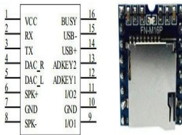
**Fig-5:** Pin configuration of MP3 module
