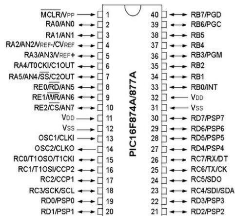
Fig -2: PIN configuration
