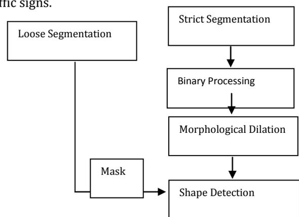
Fig-2: Work flow of detection system
