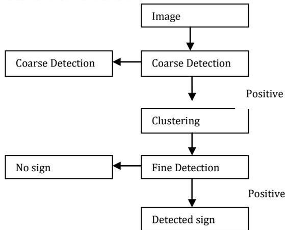
Fig-3: Step by step detection process
