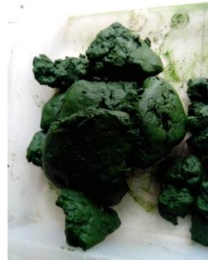
**Fig - 3:** Filtered biomass using 70 µm filter cloth.
