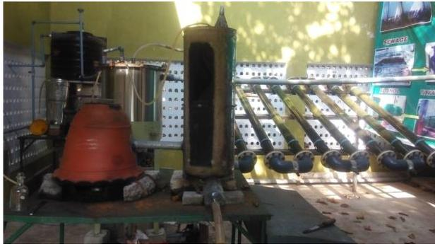
**Fig - 1:** CO<sub>2</sub> sequestration setup at the front, tubular Photobioreactor at the back.
