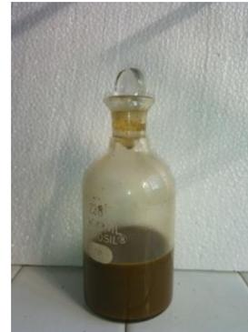
Fig - 5: Extracted lipids from dry microalgal powder
