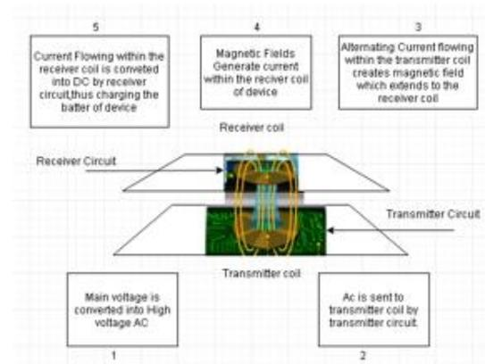
Fig 2.3: Working of wireless charging [3]
