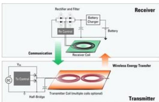
Fig 2.2: Circuit Diagram [4]
