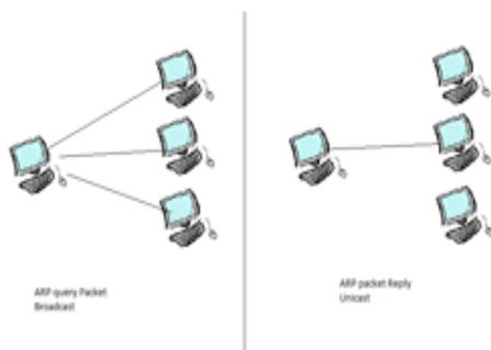
Fig 1.1.a: ARP query request Fig 1.1.b ARP reply
