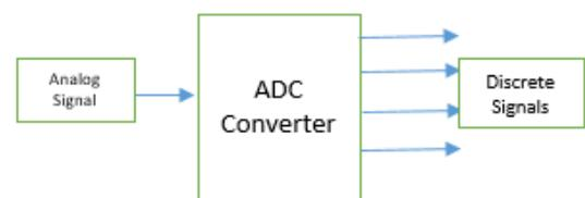
Fig 3.1.1: Block Diagram of ADC
