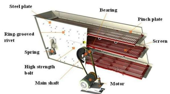
A screening machine consist of a drive that induces vibration, a screen media that causes particle separation, and a deck which holds the screen media and the drive and is the mode of transport for the vibration.
